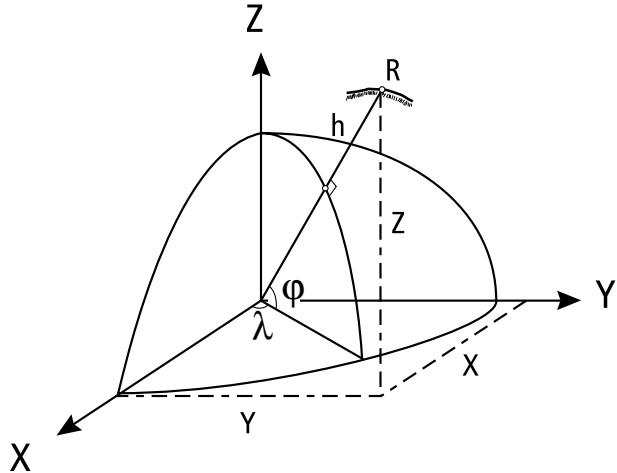
Figure 3: ECEF and Reference Ellipsoid
